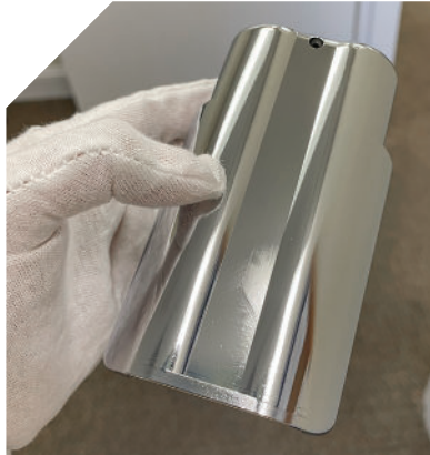
Pyramid Molding Group outsources aspects of its mold build process to experts in the necessary technology and processes. For example, this housing cover was chrome-plated by Astro Electroplating. Source | Astro Electroplating
